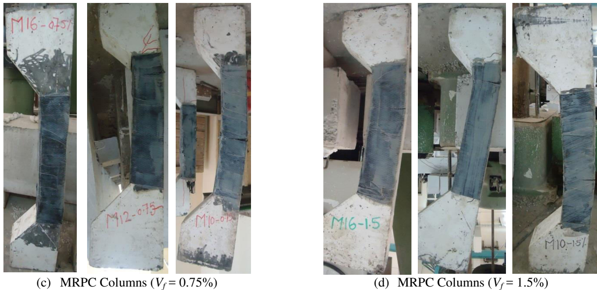
Figure (16) Strengthened Columns After Retesting
