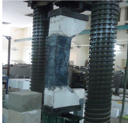
Figure (5): strengthened column under Retesting
