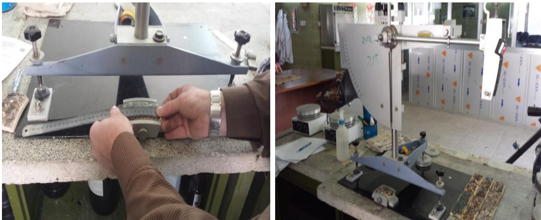
Figure 4. British Pendulum Tester
