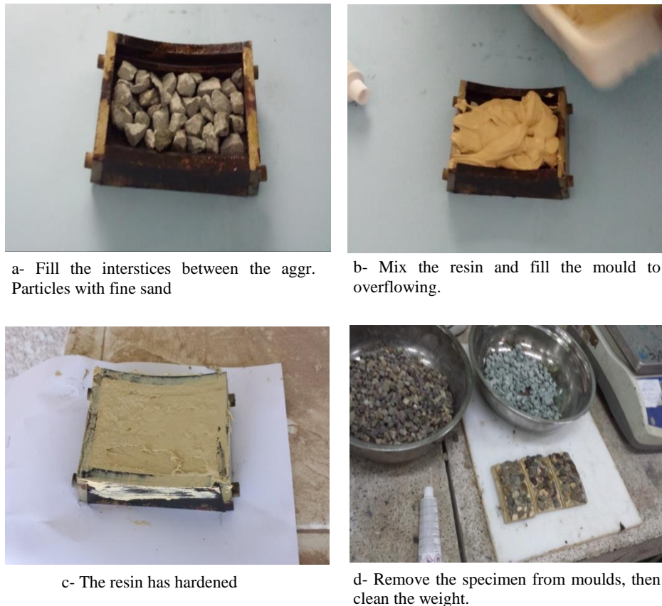
Figure 2. Procedure for Sample Preparation Prior To Testing
