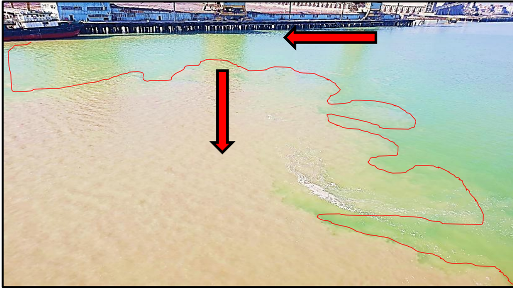
Figure 9. The penetration of suspended materials into the channel has stopped near the silo quay at the highest tide. The red line is bordering the accumulated fresh sediment. Depth was measured using the Echo Sounder device. Location: 30°02'32.0"N, 47°56'49.3"E. Photo date: 8/12/2020.
