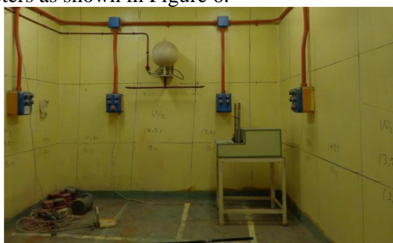
Figure 6. Grids distribution ceilings, walls and floor of rooms in the radiochemistry laboratory building.
