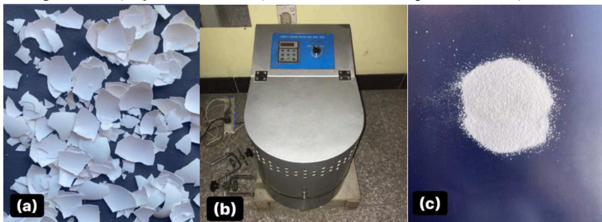
Figure 1. a) crushed eggshell b) milling device c) ground eggshell
