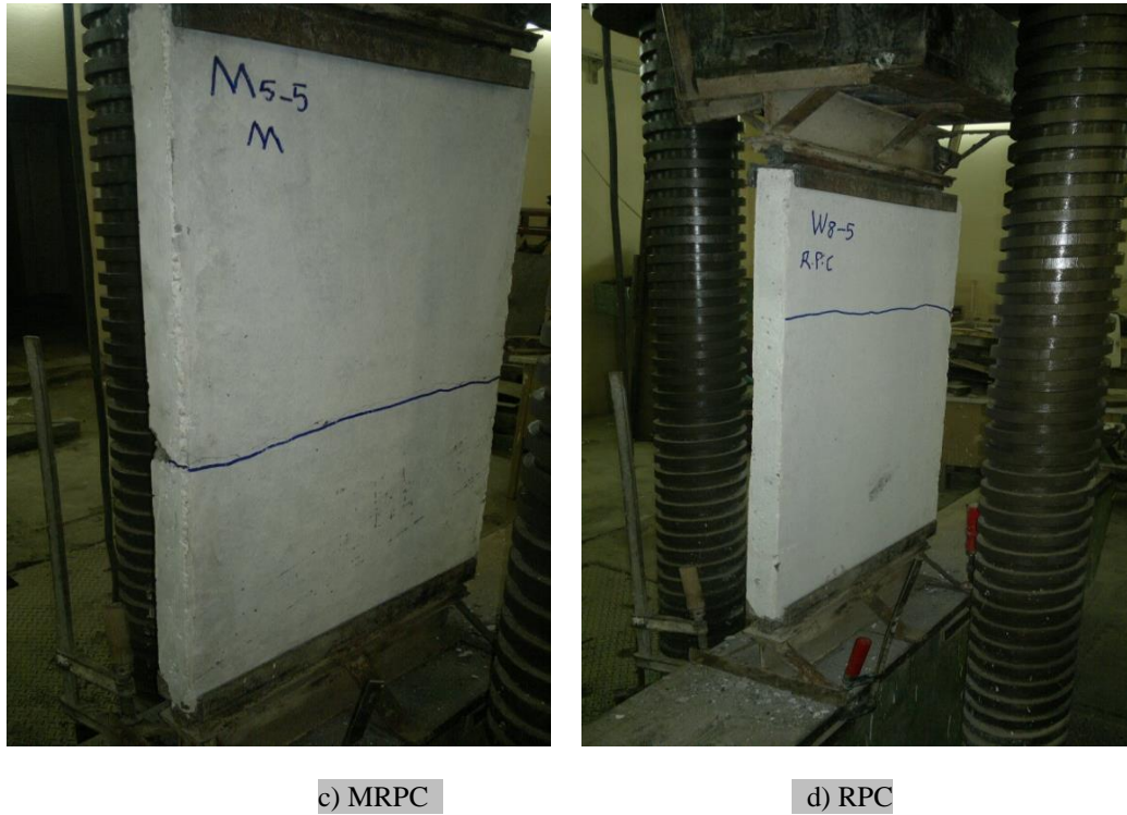
Fig(13)Crack pattern for panels with H/t=14
