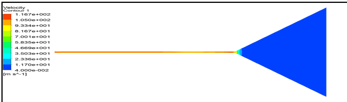
Figure (11): Contour of velocity distribution for smooth cone (without rib) with at air velocity 0.04 m/s
