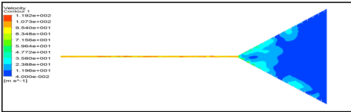
Figure (12): Contour of velocity distribution for cone with spiral square rib at inlet air velocity 0.04 m/s
