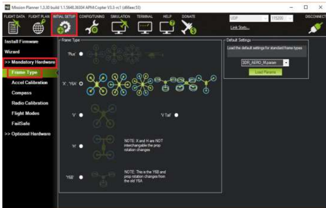
Figure (7) Mission Planner that selects UAV frame type
