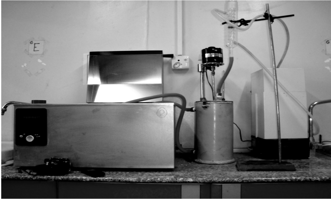
Fig .(2) Photographic picture of the chlorophyll extraction experimental apparatus
