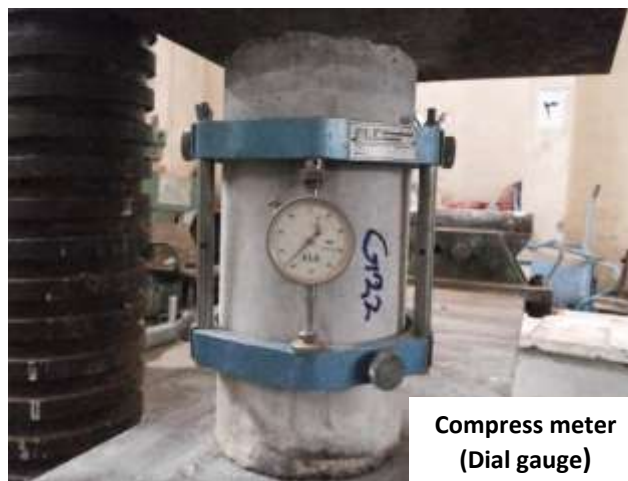
Plate8. Modulus of elasticity test of concrete specimens
