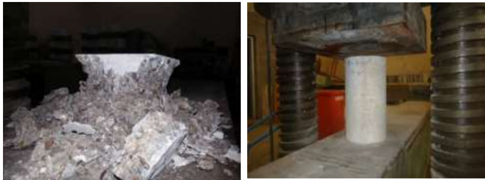
Plate 5. Test of compressive strength of concrete
