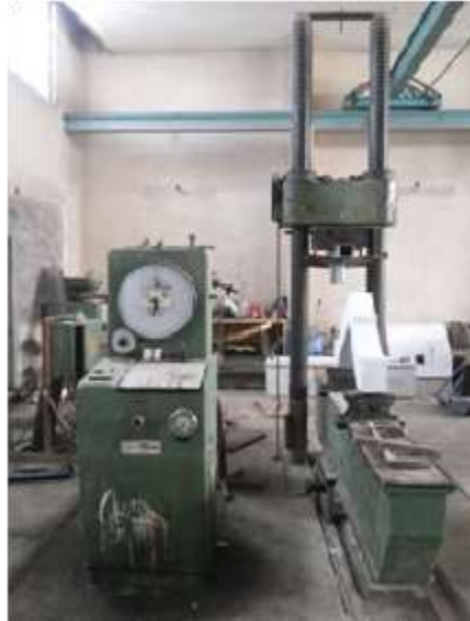
Plate 3. Universal testing machine (MFL System) used in this work.
