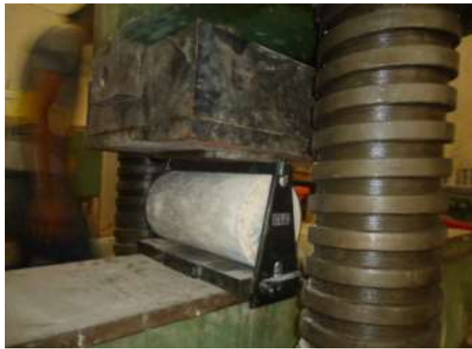
Plate 6. Splitting tensile test of concrete
