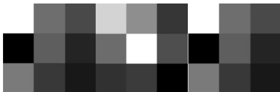
Fig. 1. Image blocks in ex.2 & ex.3. Left: original image f(x,y) . Middle: blurred g(x,y) . Right: estimated image \hat{f}(x,y) .
