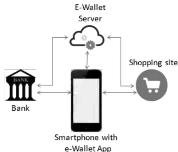
Fig. 1. Components in e-wallet service.
