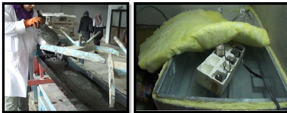
Plate .(1): casting and curing of specimens
