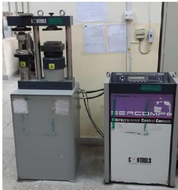
Fig.4. Universal compressive machine(Sercomp, Controls Co.) Italy.
