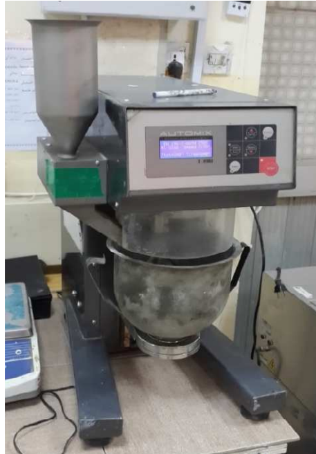
Fig.2 Electrical mixer (Automix, Controls Co. Italy)
