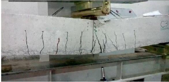
Plate (8) Crack pattern of C3 specimen
