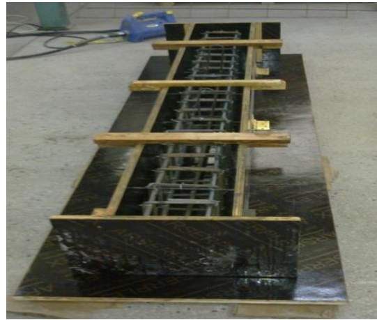
Plate (2) Top view of mold and reinforcement
