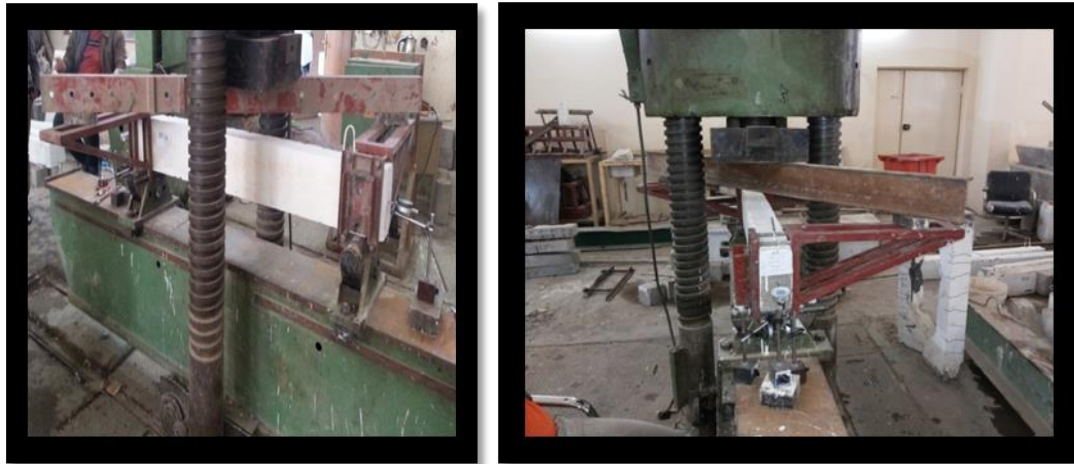
Figure (6): Arrangement of Beam Testing
