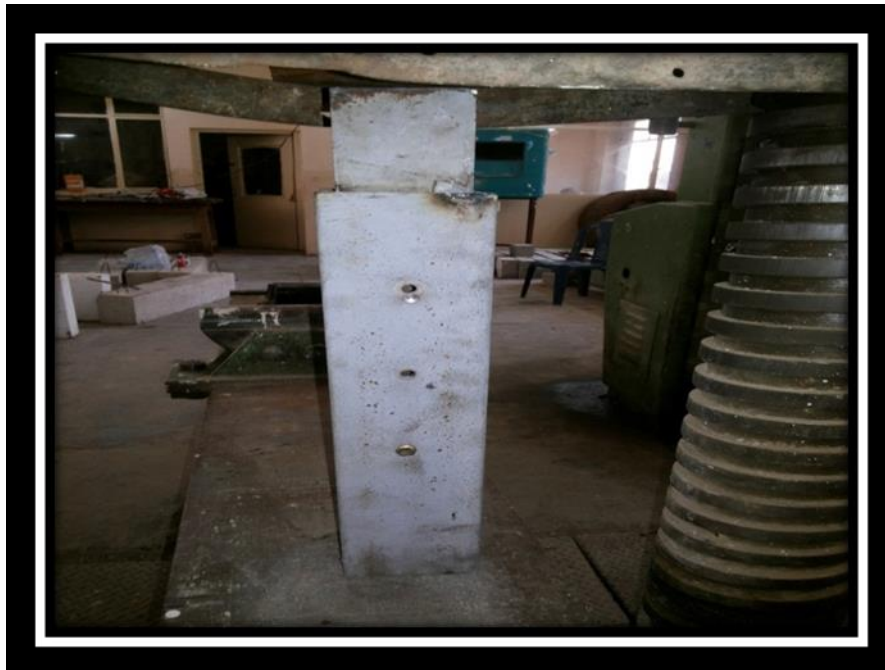
Figure (4) The direct- shear strength test
