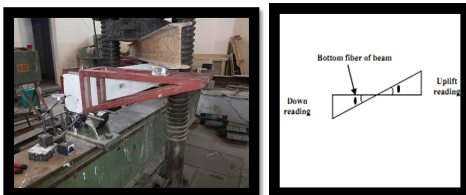
Figure (7): Angle of Twist Measurement
