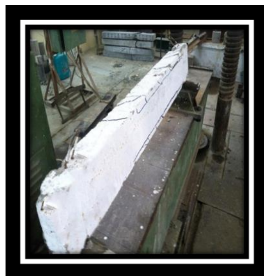
Figure (15): Crack Pattern and Failure Composite beam (B3)
