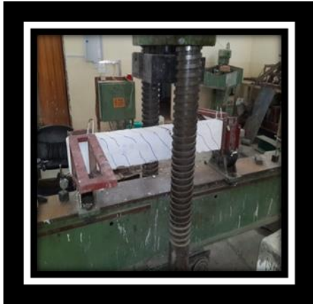
Figure (12): Failure of Reference (BN) Specimen
