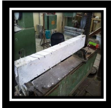
Figure (13): Crack Pattern and Failure Mode of composite beam (B1)
