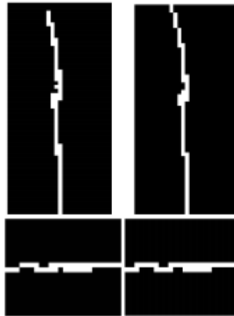
Fig .4. Example of defect binarization
