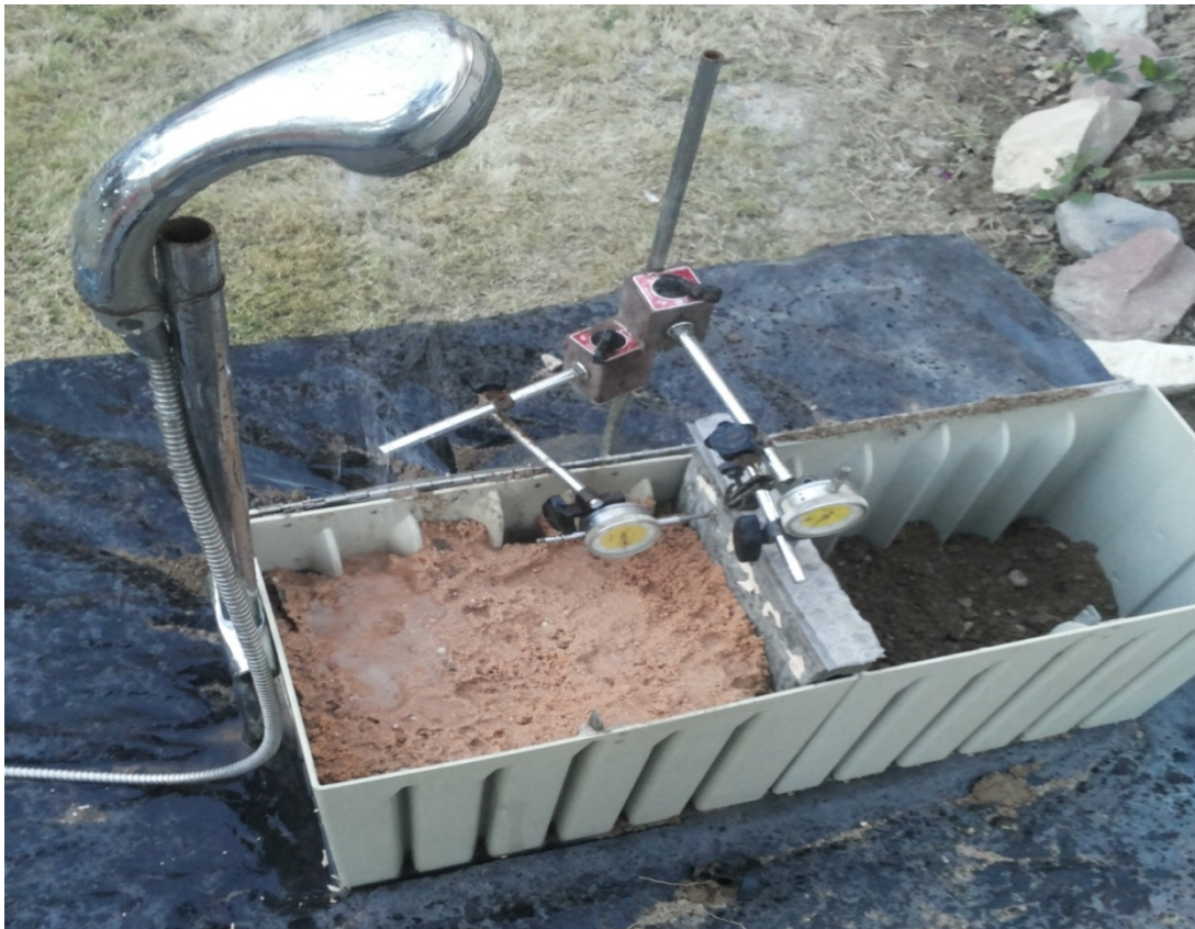
Fig .(6) wetting of soil by feeding water from a sprayer device, and starting test by taking the vertical and horizontal displacement with time.
