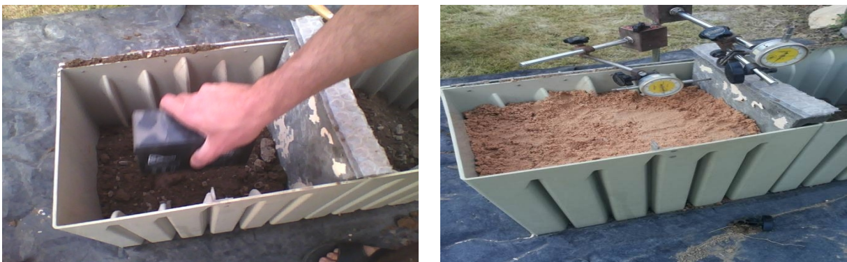
Fig .(5) preparation steps for the bed gypseous soil ,Compaction natural gypseous soil bed and placement of sand backfill and dial gauges fitting.
