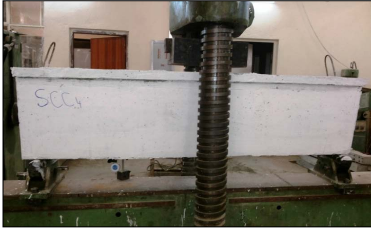
Figure (2): Beam Specimen Setup.
