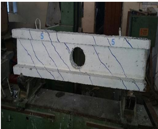
Figure (25): Crack pattern and modes of Failure (B5)
