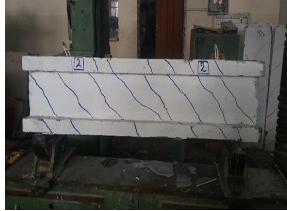
Figure (22): Crack pattern and modes of Failure(B2)
