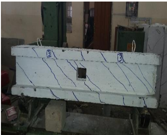
Figure (23): Crack pattern and modes of Failure (B3)
