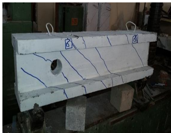
Figure (26): Crack pattern and modes of Failure (B6)
