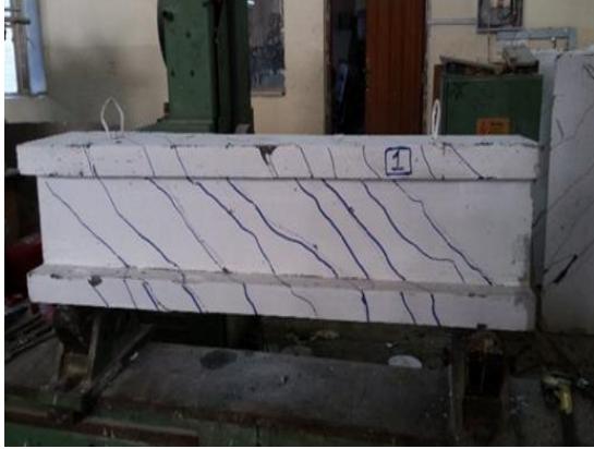
Figure (21): Failure of Reference (B1)
