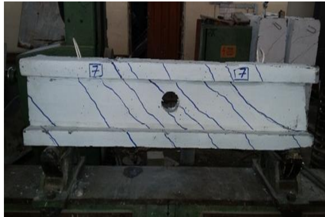
Figure (27): Crack pattern and modes of Failure (B7)
