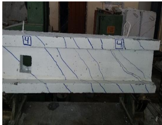
Figure (24): Crack pattern and modes of Failure (B4)
