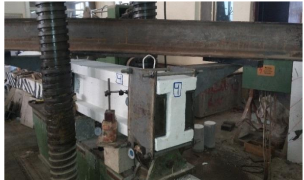
Figure (4): Arrangement of Beam Testing
