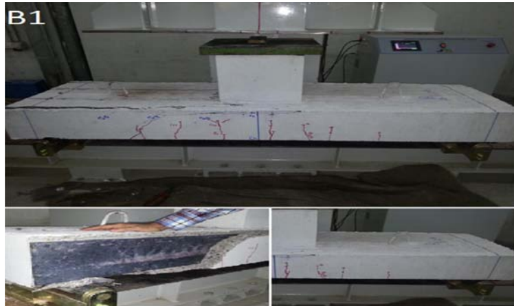
Figure (7) Crack pattern for (B1)
