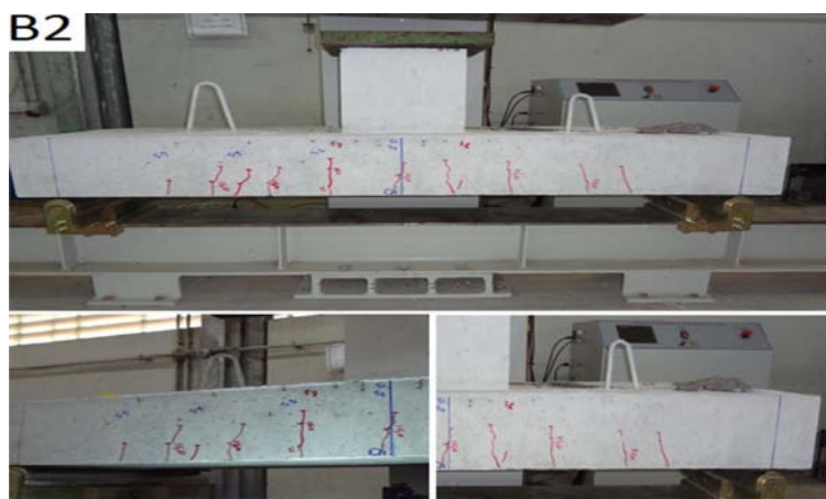
Figure (8) Crack pattern for (B2)
