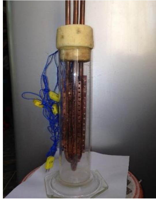
Figure (7) Capsule with two copper U tube with perforated longitudinal fins
