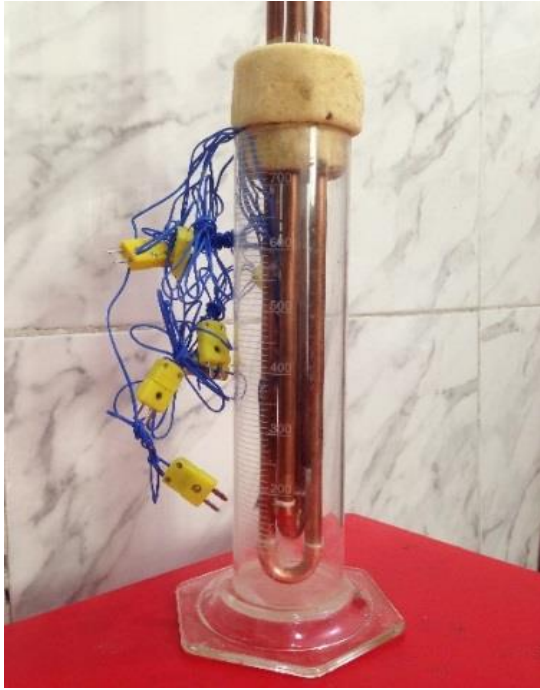
Figure (6) Capsule with two copper U tube
