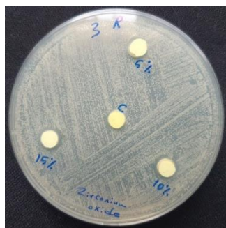
Figure (2): The Agar-Well diffusion test for the susceptibility of Candida albicans Isolate to alginate impression material incorporated with different concentrations of zirconium oxide nanoparticles.
