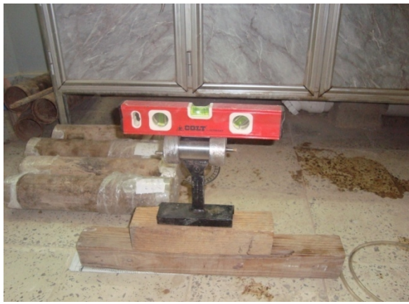
Plate .(11) Use of manual water bubble for ensuring the device horizontally.
