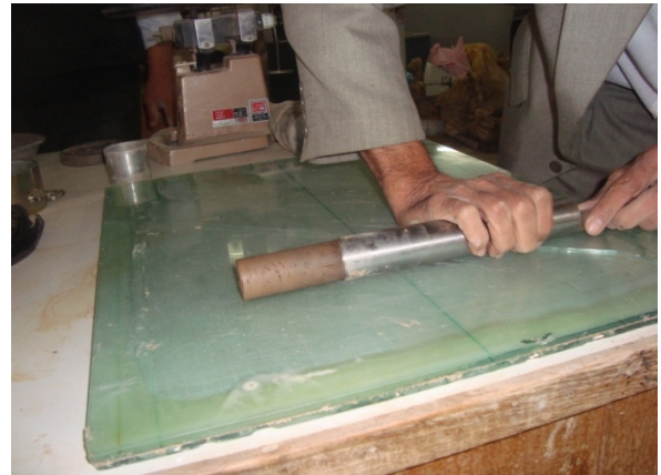
Plate .(4) Extracting the sample of sampling tube.
