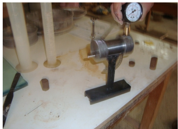
Plate .(10) Connecting the top cover and the pressure gauge.
