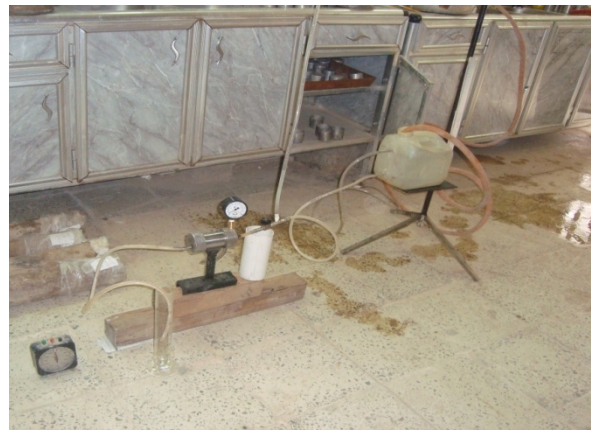
Plate .(12) The use of a mobile water tank for achieving hydraulic head.
