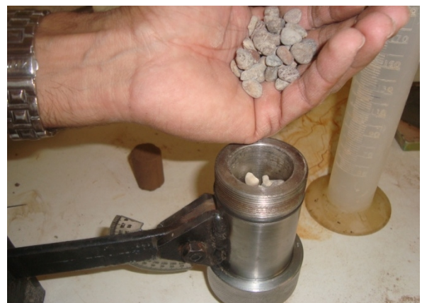
Plate .(6) Putting a layer of fine gravel at bottom of the sample.
