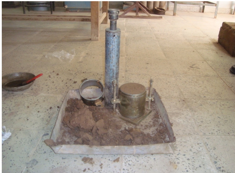
Plate .(2) Preparation of sample by the standard compaction device.
