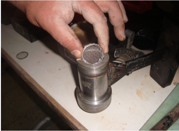
Plate .(7) Circular wire mesh No. (2) above the layer of fine gravel.
