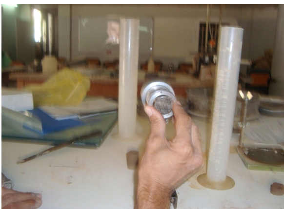
Plate .(9) introduction of circular wire mesh No. (1) above the clayey sample.
