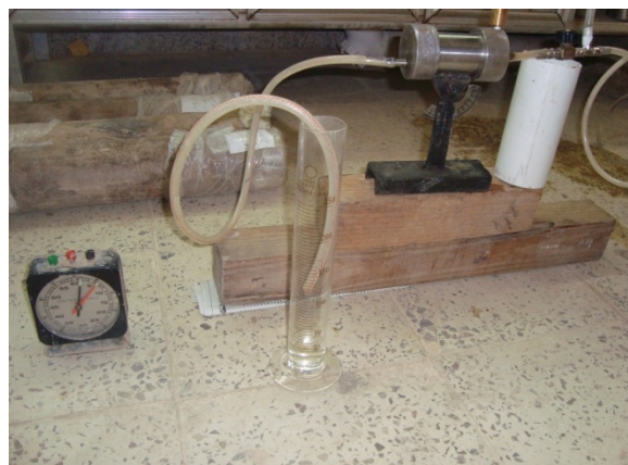
Plate .(13) Assembling the water leaving the model in a graduated cylinder and recording time.
