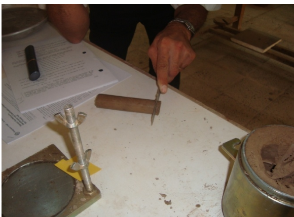
Plate .(3) Extraction of the desired measurement model using tube-making for this purpose.
