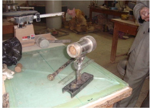
Plate .(8) Insertion of conical ring inside the clayey sample.
