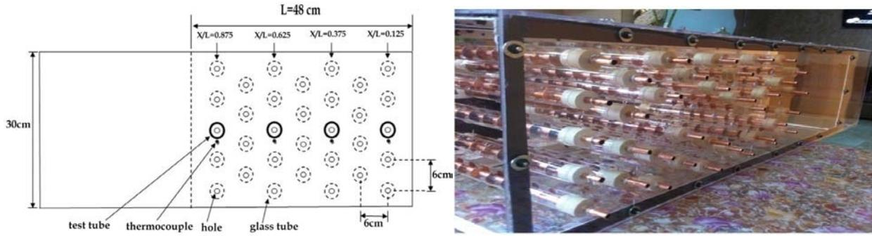
Figure (3): Double-tubes arrangement of the FWD system.
