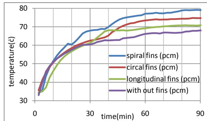
**Figure (13): PCM transient temperature response for each type of WD recovery systems during charging process.**
