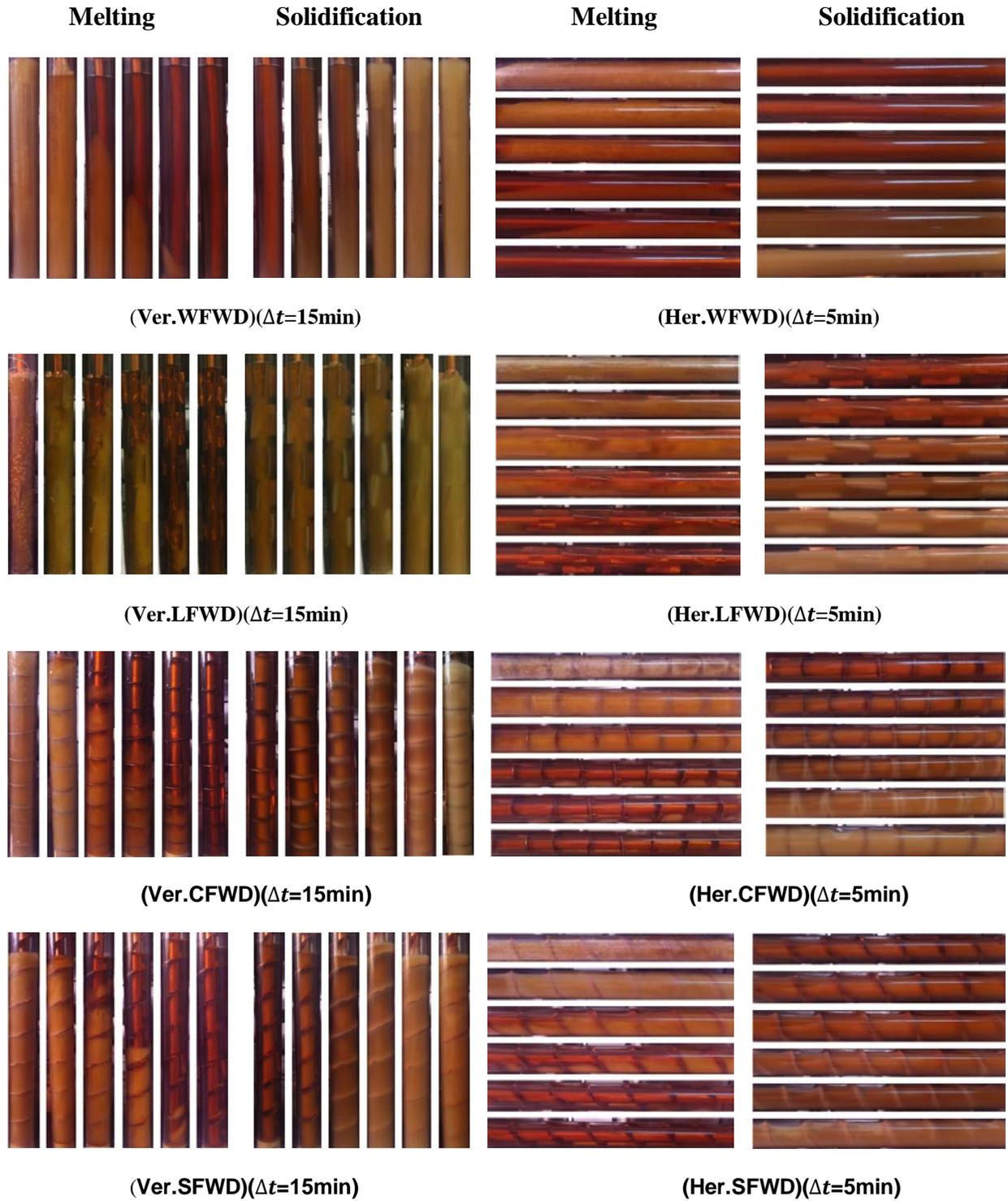
Figure (11): Propagation of melting and solidification fronts of PCM with different types of fin profiles.
