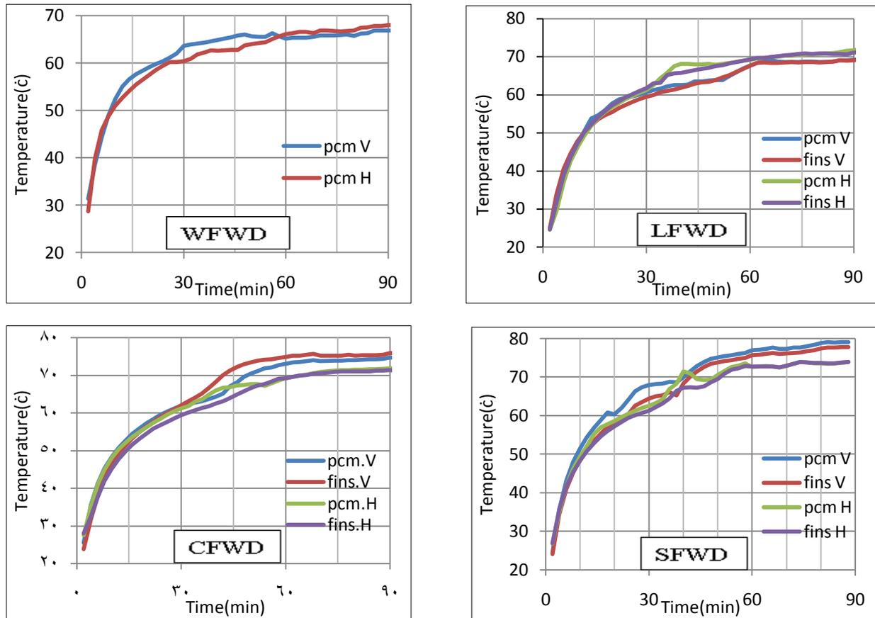
**Figure (16): Comparison between vertical and horizontal position thermal response inside WD recovery system**
