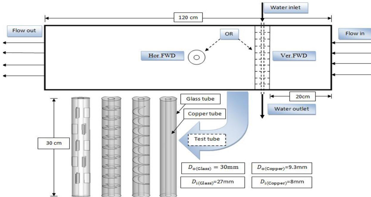
**Figure (1): Physical representation of the FWD system**
