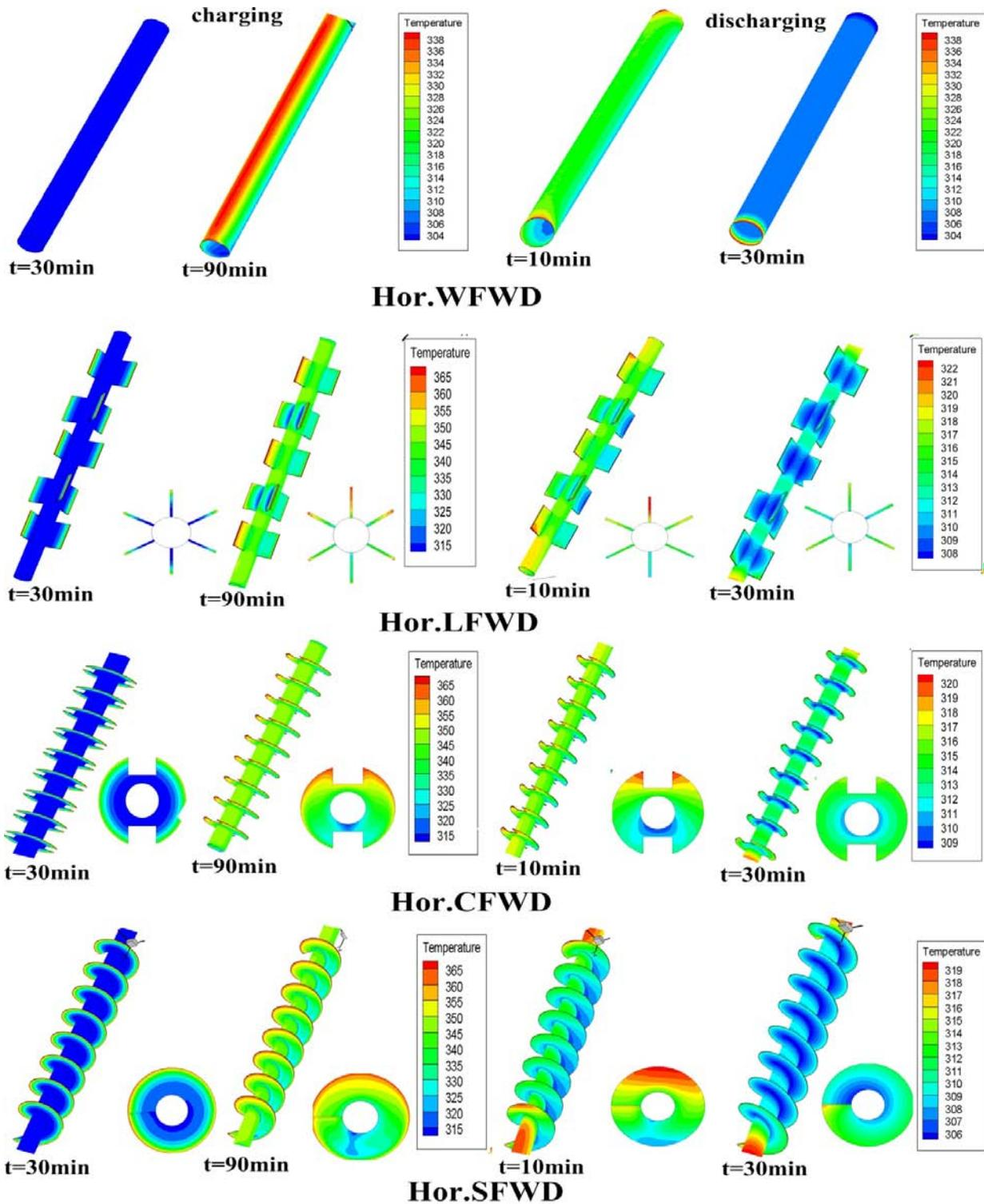
Figure (9): Transient temperature contours of PCM inside horizontal vertical FWD systems.
