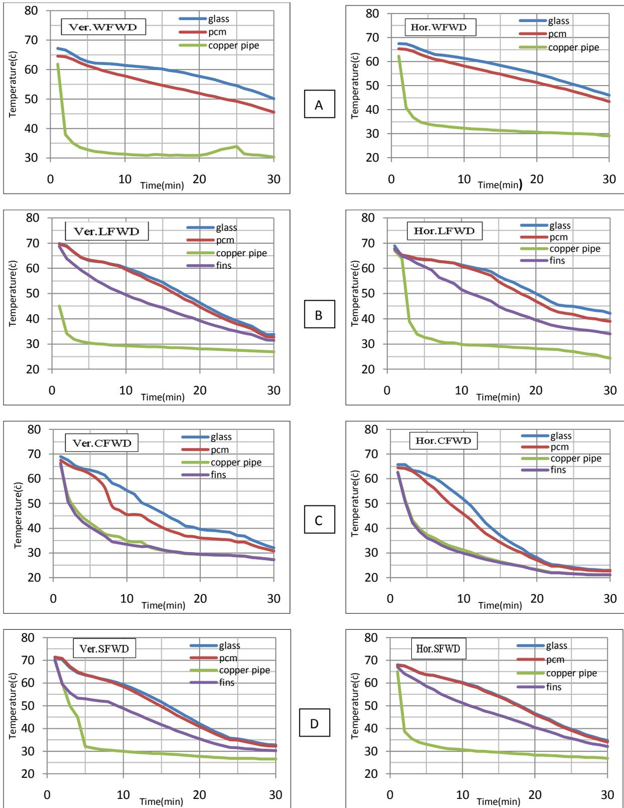
**Figure (15): Measured radial temperature distribution inside WD systems during discharging process.**
