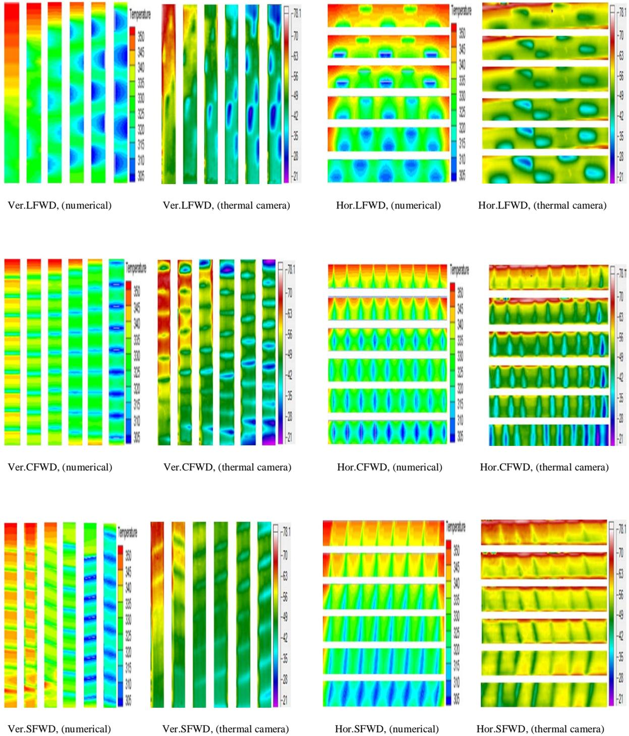
**Figure (12): Comparison between the results of ANSYS numerical software with photos of thermal camera for single FWD during discharging process. ( $\Delta t = 5\text{min}$ )**
