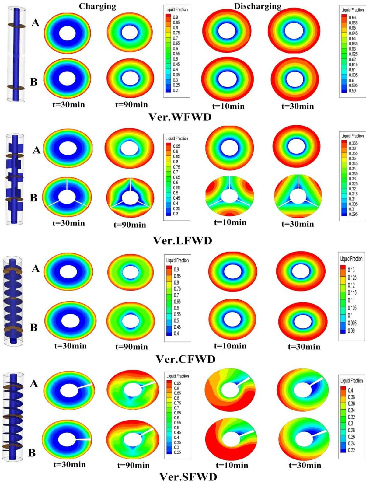
Figure (6): Transient liquid fraction contours of PCM inside various vertical FWD systems.
