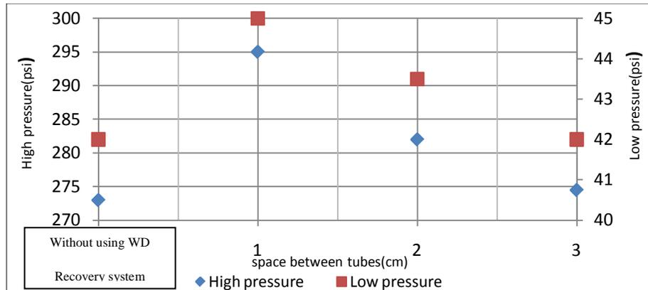
**Figure (5): Effect of space between tubes of the WD system on low and high pressure of the air conditioning unit.**
