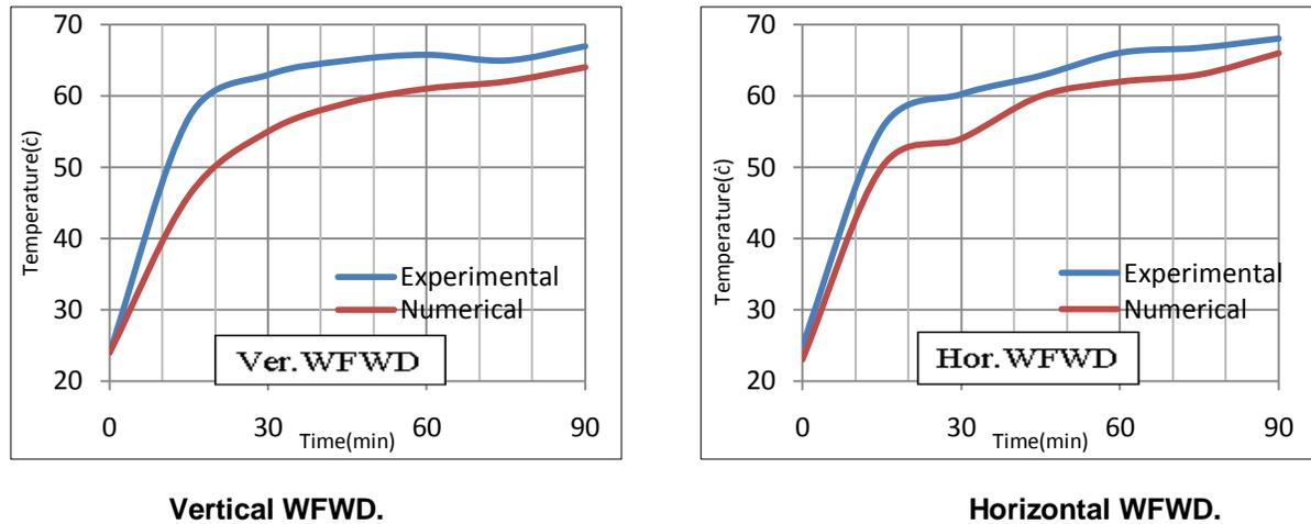
**Figure (10): Comparison between experimental and numerical results for WFWD system during melting process**
