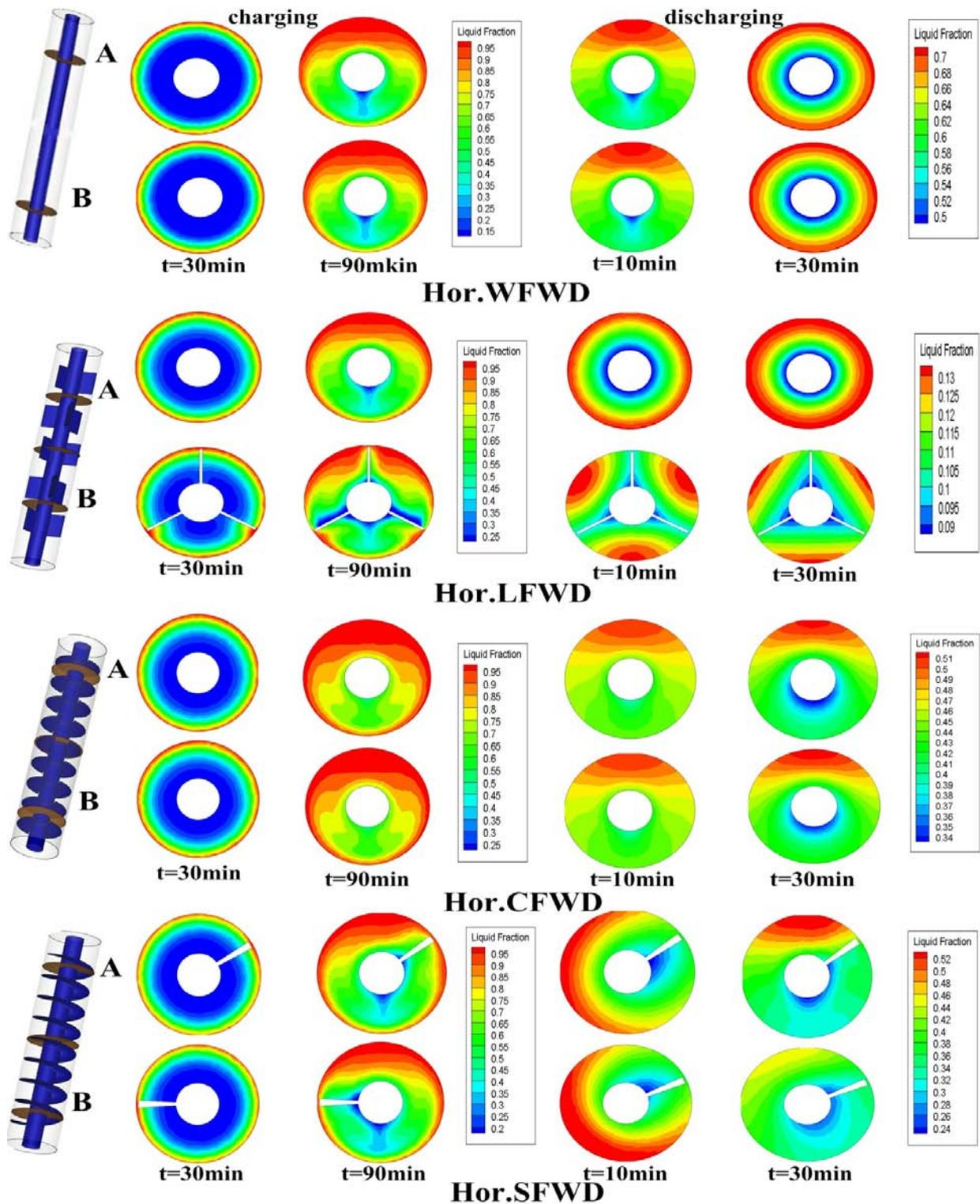
Figure (7): Transient liquid fraction contours of PCM inside various horizontal FWD systems.
