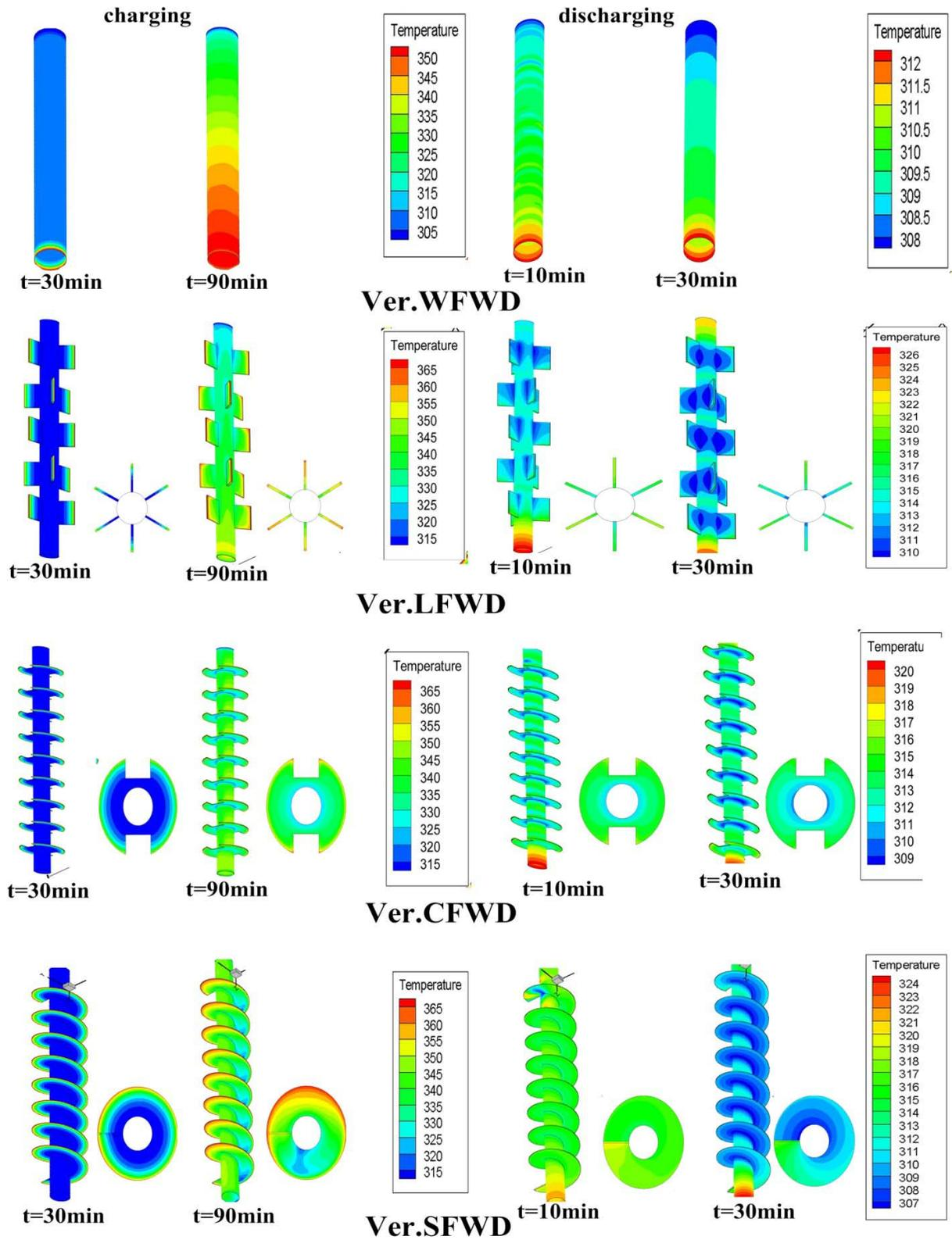
Figure (8) Transient temperature contours of PCM inside various vertical FWD systems.
