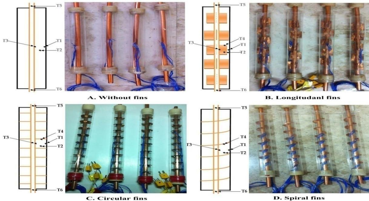
Figures (4): Thermocouples positions of the test tubes.
