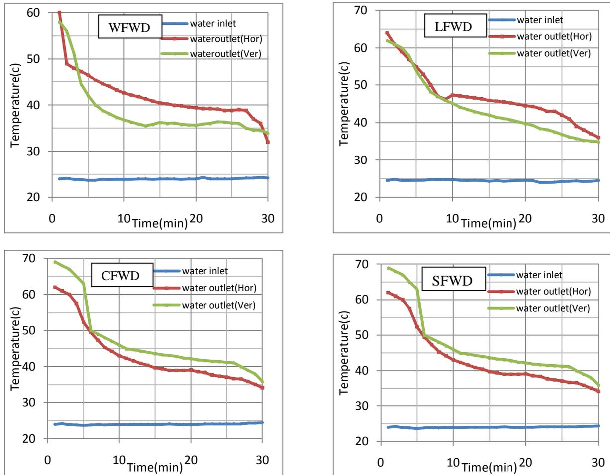
**Figure (17): Transient water temperature during discharging process for FWD systems.**
