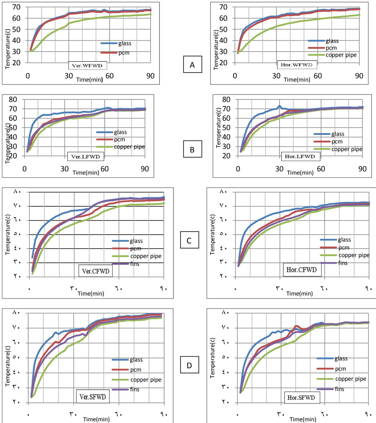
**Figure (14): Measured radial temperature distribution inside WD systems during charging process.**
