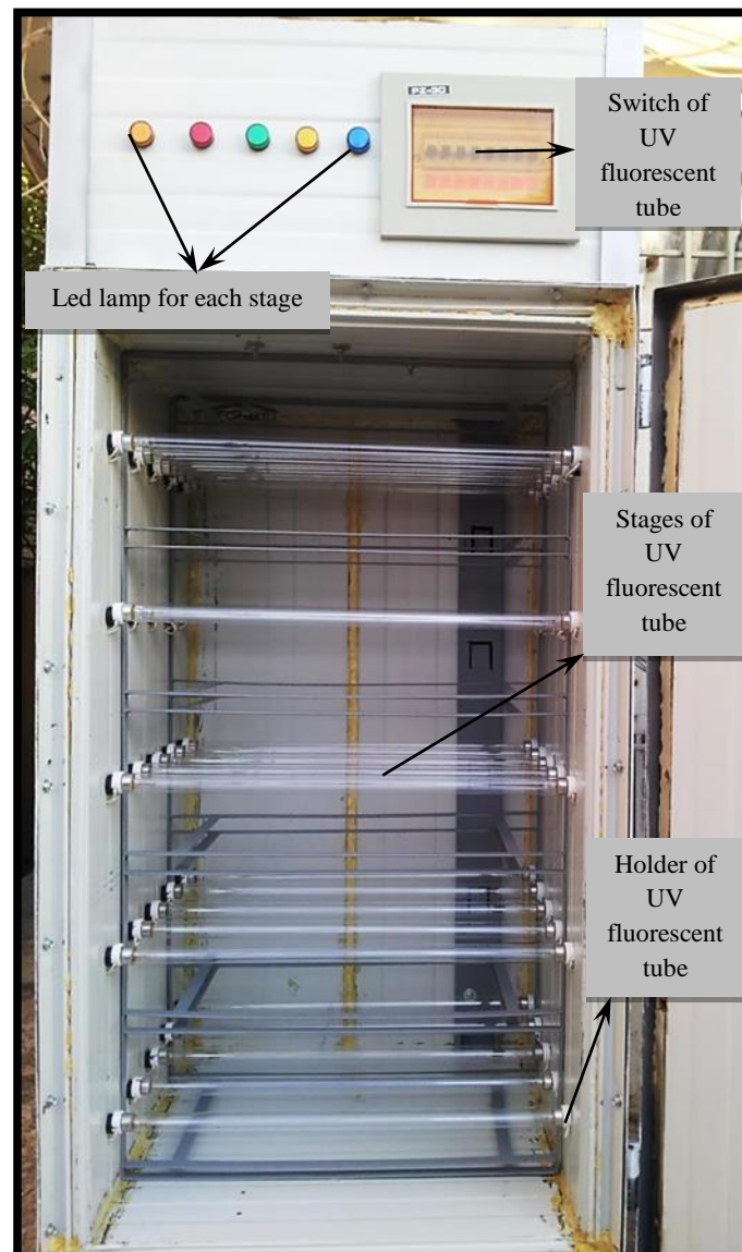
Figure (9) Arrangement of UV fluorescent tube.
