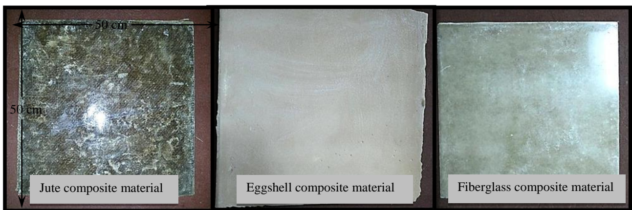
Figure (5) Specimens of jute, eggshell and fiberglass composite material.
