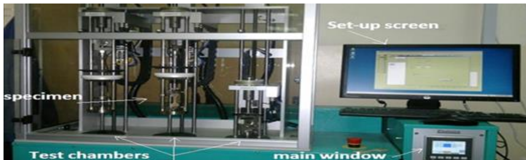
Figure7. Device of creep/stress relaxation test.
