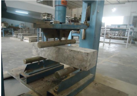
Fig .(7) Flexural strength test
