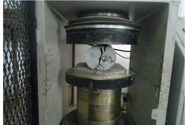
Fig .(8) Splitting tensile strength test
