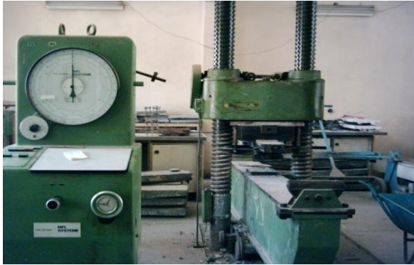
Fig .(9) Flexure testing machine
