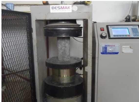
Fig .(5) Compressive strength test
