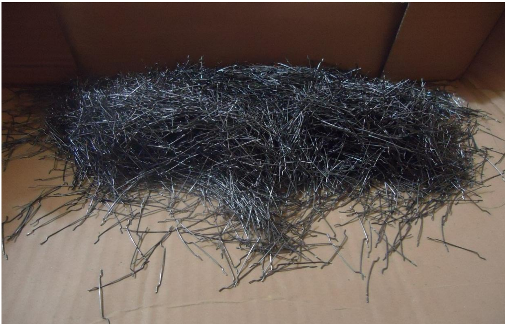
Fig .(2) Sample of the used steel fibers
