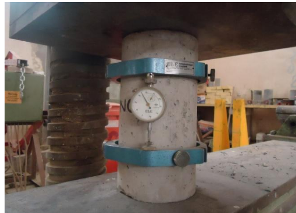
Fig .(6) Modulus of elasticity test
