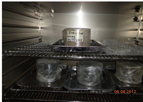
Fig .(6) Curing Condition for Samples Treated with Lime-silica fume.
