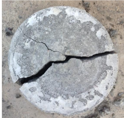
Fig .(11) Failure crack for cylindrical specimen mixture C5
