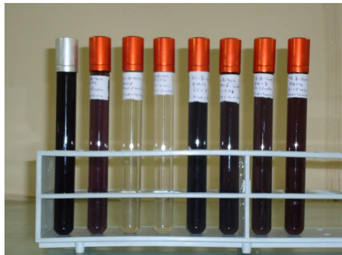
Figure 4. Effect of pH variation (from left to right - raw effluent; treated effluent with pH value, 2; 3; 4; 5; 6; 8; and 10, respectively)
