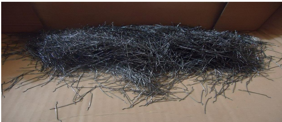
Fig .(2) Sample of the used steel fibers
