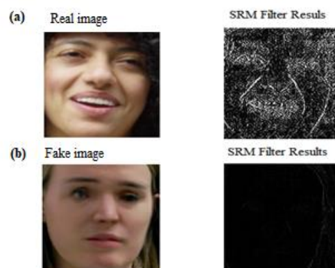
FIG.3. APPLYING SRM FILTER ON FAKE AND REAL IMAGES. (A) AN EXAMPLE OF APPLYING SRM FILTERS TO THE REAL IMAGE. (B) THE RESULTS OF APPLYING SRM FILTERS ON THE FAKE IMAGE.
