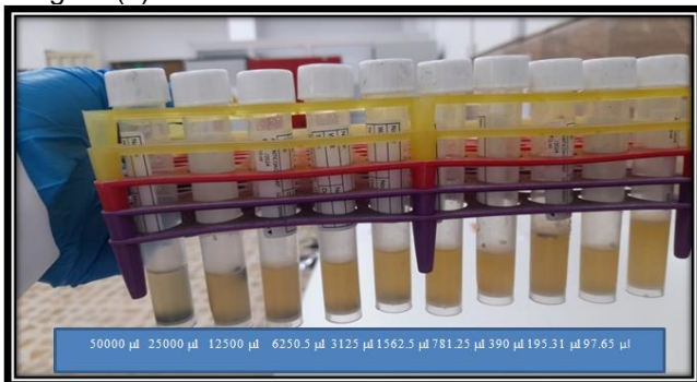
Figure (3): Serial dilution method for detection of the MIC of silver nanoparticles against K. pneumoniae sub-Spp pneumonia
