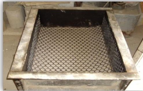
Plate No. (9): Folding GG2 Geogrid in 90° against the Long Side of Steel Container.
