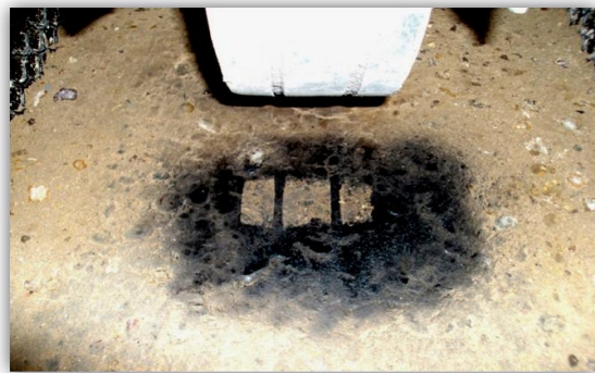
Plate No. (2): Contact Area between Tire and Subbase.
