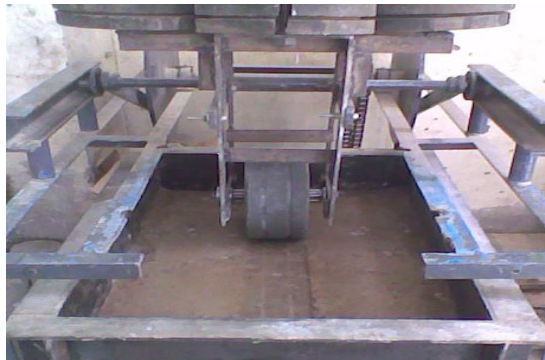
Plate No. (10): Coinciding Wheel with the Center of the Subbase Surface.
