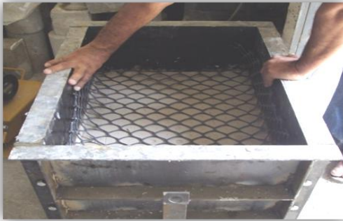
Plate No. (8): Folding GG1 Geogrid in 90° against the Long Side of Steel Container.
