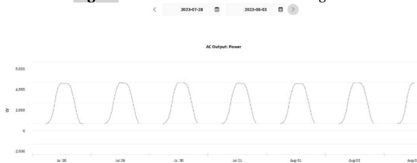
Fig. 11 The PV Monitor AC Output Power Display.
