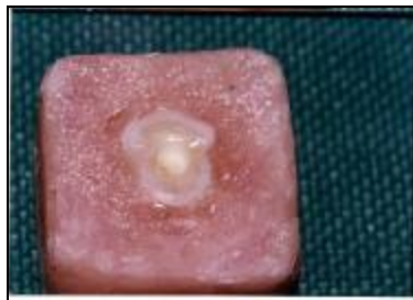
Figure 2: Sample after cavity preparation
