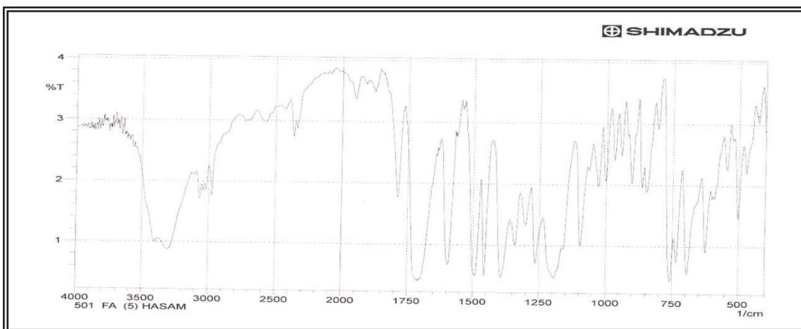
(Figure 2): FT-IR spectrum of compound B2
