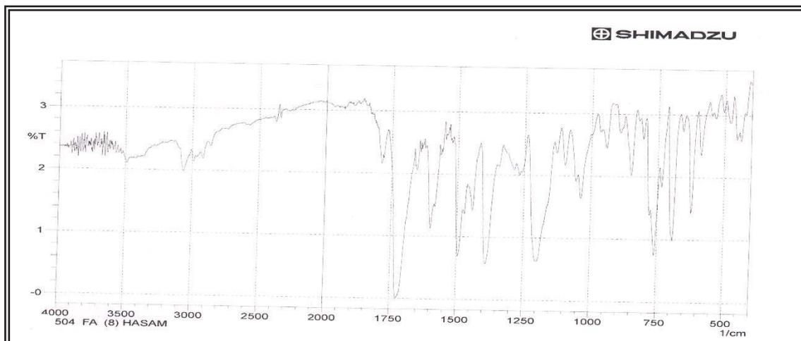
(Figure 1): FT-IR spectrum of compound B1
