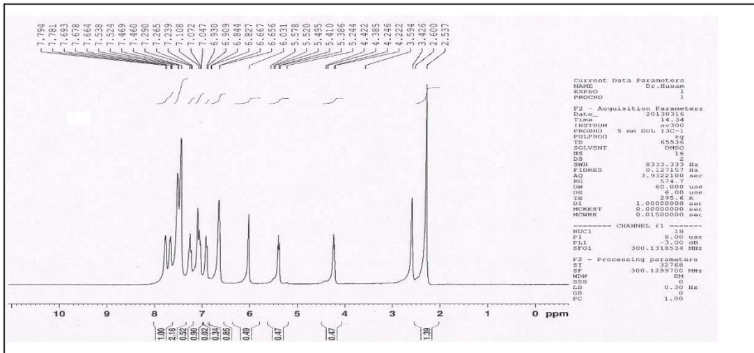
(Figure 4): <sup>1</sup>H-NMR spectrum of compound B1
