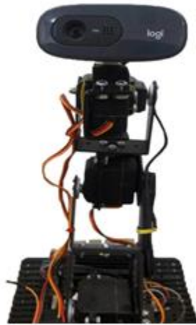
FIG. 4. LOGITECH C270 CAMERA USED IN RESEARCH.
