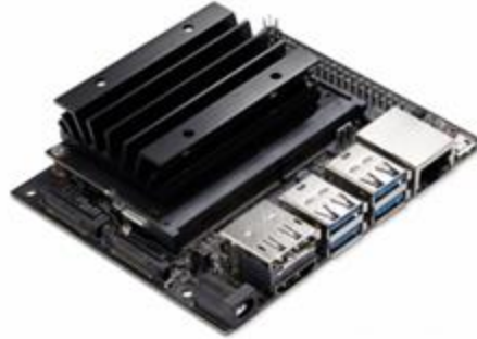
FIG. 6. JETSON NANO DEVELOPER KIT BOARD.
