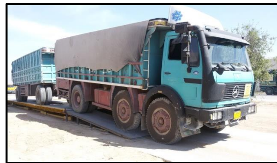
(f) Weighing the trailer unit alone ( W_2 ).
