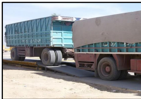
(g) Weighing the rear axle of the trailer ( R_2 ) alone.
