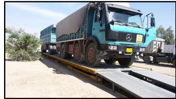
(d) Weighing the whole vehicle (tractor and trailer) ( W_t ).
