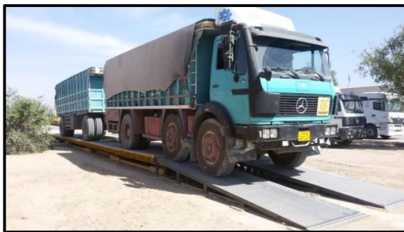
(e) The front axle of the tractor outside the platform.
