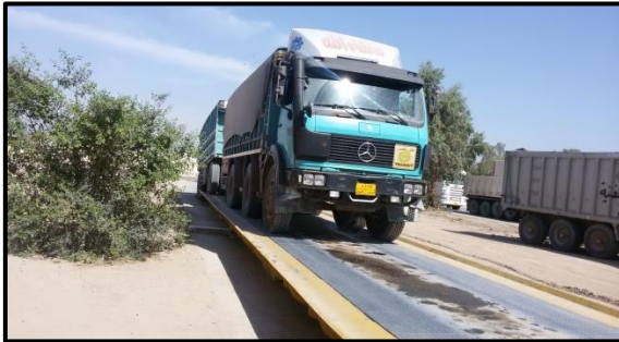
(c) Weighing the tractor's axles together with the front axle of the trailer
