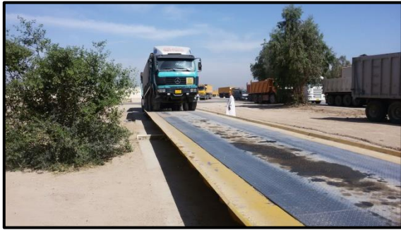
(a) Weighing the front tandem axle ( F_1 ) of the tractor alone.
