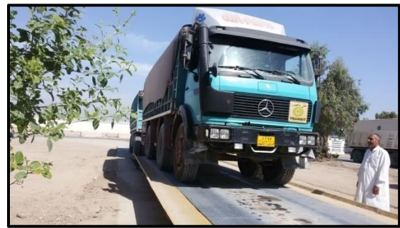
(b) Weighing all axles of the tractor together ( W_1 ).
