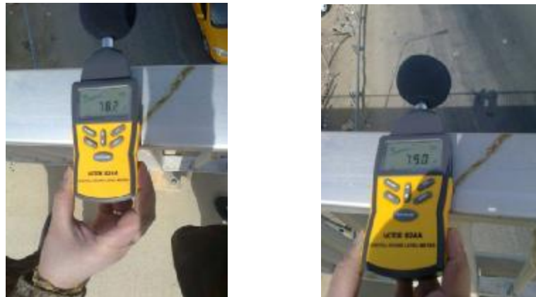
Fig. (2) Digital Sound Level Meter (Victor 824 A)
