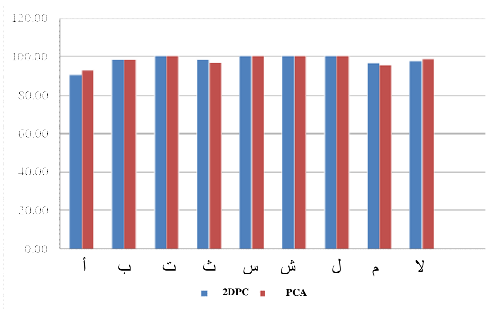
Fig. (6); The recognition rate of PCA and 2DPCA classifiers using 405 training samples
