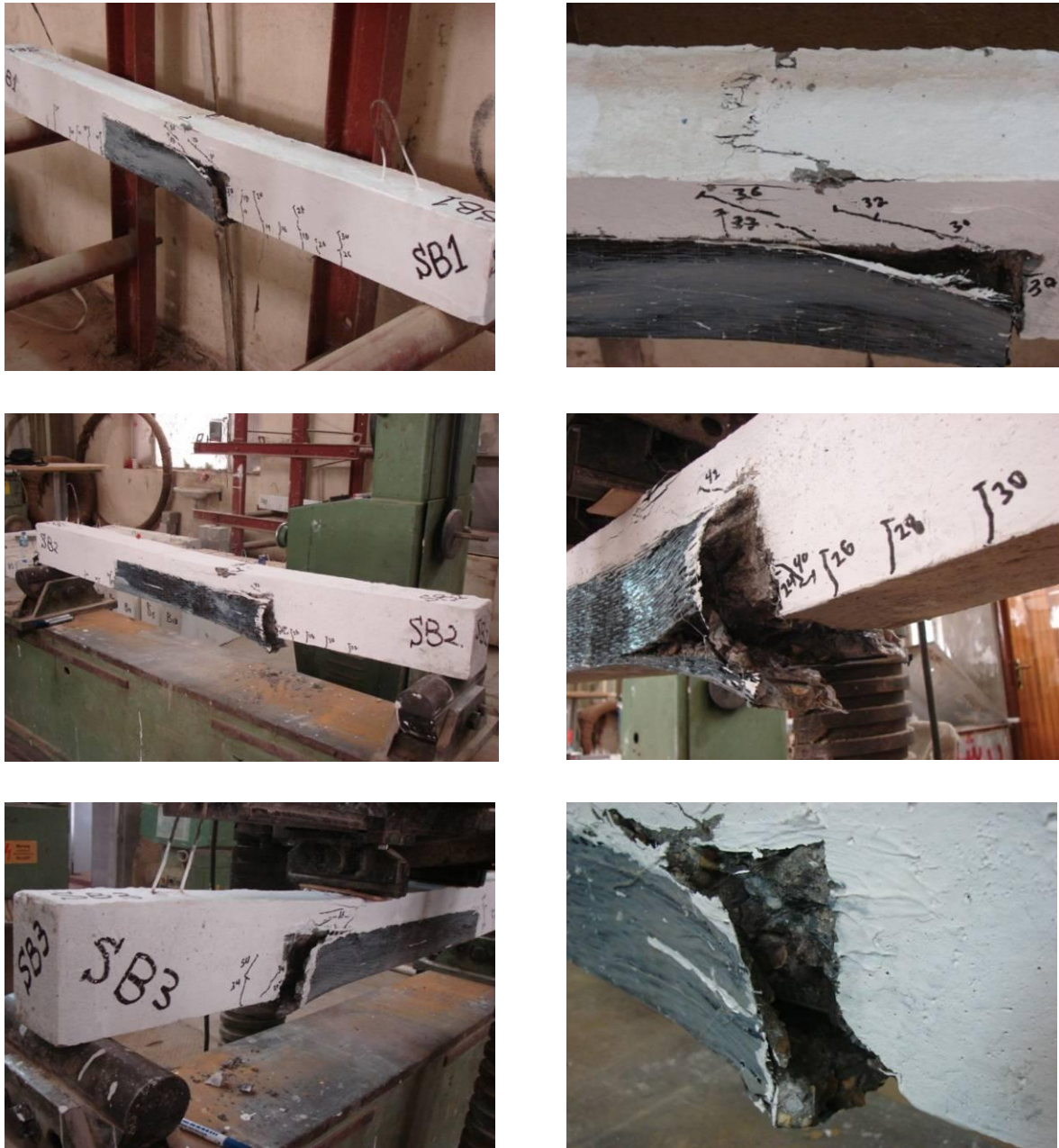
Figure (6) shows the beams crack and failure type
