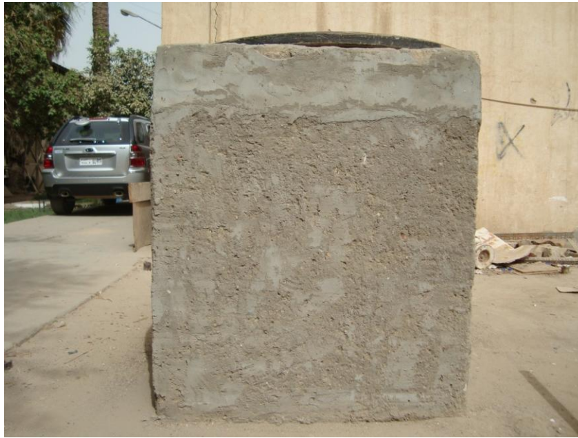
Fig (1) The room is built of brick (0.12m) thickness and coated by cement layer (0.002m) thickness
