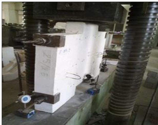
Figure (12) Dial Gauges to Measure Lateral Movement
