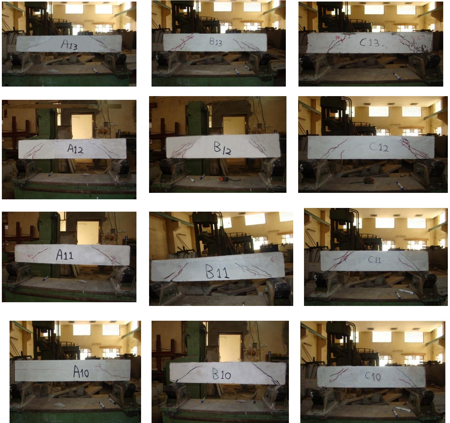
Fig (11) crack pattern of SCC beams
