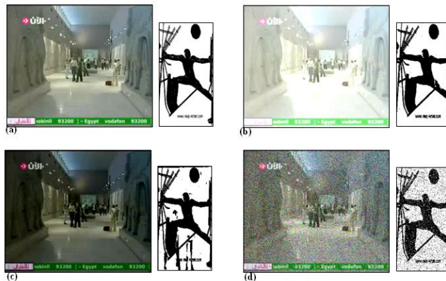
Figure (6) some type of attacks a) Original watermark and key-frame b) Lightened frame and retrieved watermark. c) Darken frame and retrieved watermark d) Noise frame and retrieved watermark.
