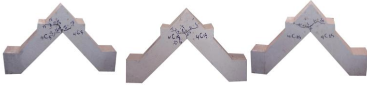
Figure (7), Failure Shape for Corners (4C5, 4C15, 4C25).
