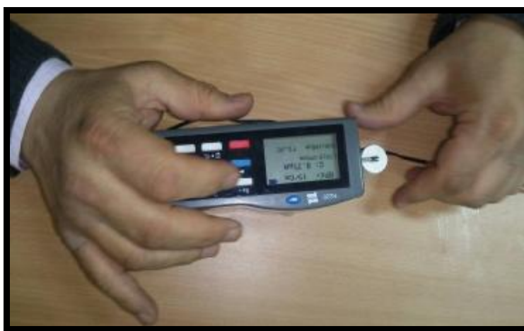
Figure (8): The surface roughness of the samples was measured with Profilometer.
