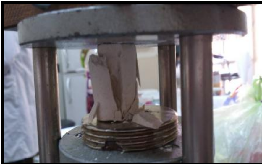
Figure (7): Specimen's fracture.
