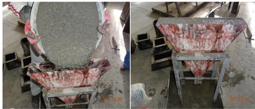
Figure (3). V-funnel test.
