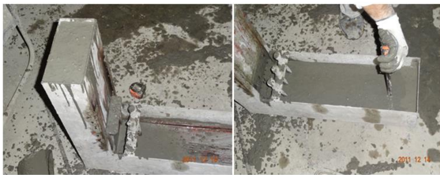
Figure (4). L-Box test.
