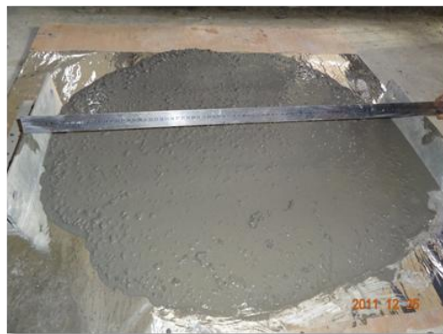
Figure (2) slump flue test.
